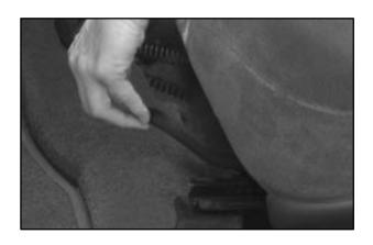
Lift the lever on the front of the driver's seat to unlock it. Slide the seat to where you want it. Then release the lever and try to move the seat with your body, to make sure the seat is locked into place.
